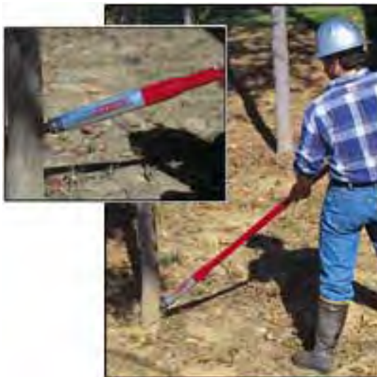
Figure 7. The EZ-ject ® lance is can be an efficient means of controlling larger shrubs and trees without non-target impacts. Photos ©2003 Forestry Suppliers, Inc. All rights reserved. Used by permission. 540010.
