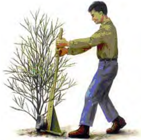
Figure 10. A Weed wrench can be an effective means of controlling shrub/tree seedlings and saplings. Illustration reproduced with permission from Brooklyn Botanic Garden.
