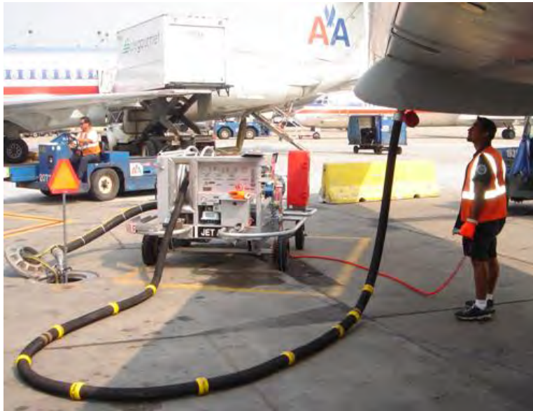
Figure 21: Hydrant Aircraft Fueling Operation 11
