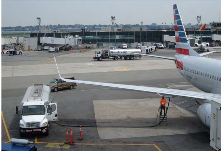
Figure 22: Bowser Fueling Operation
