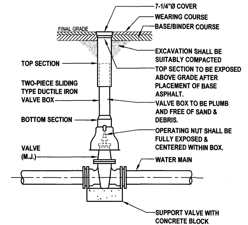
3 Valve Box Installation Detail
