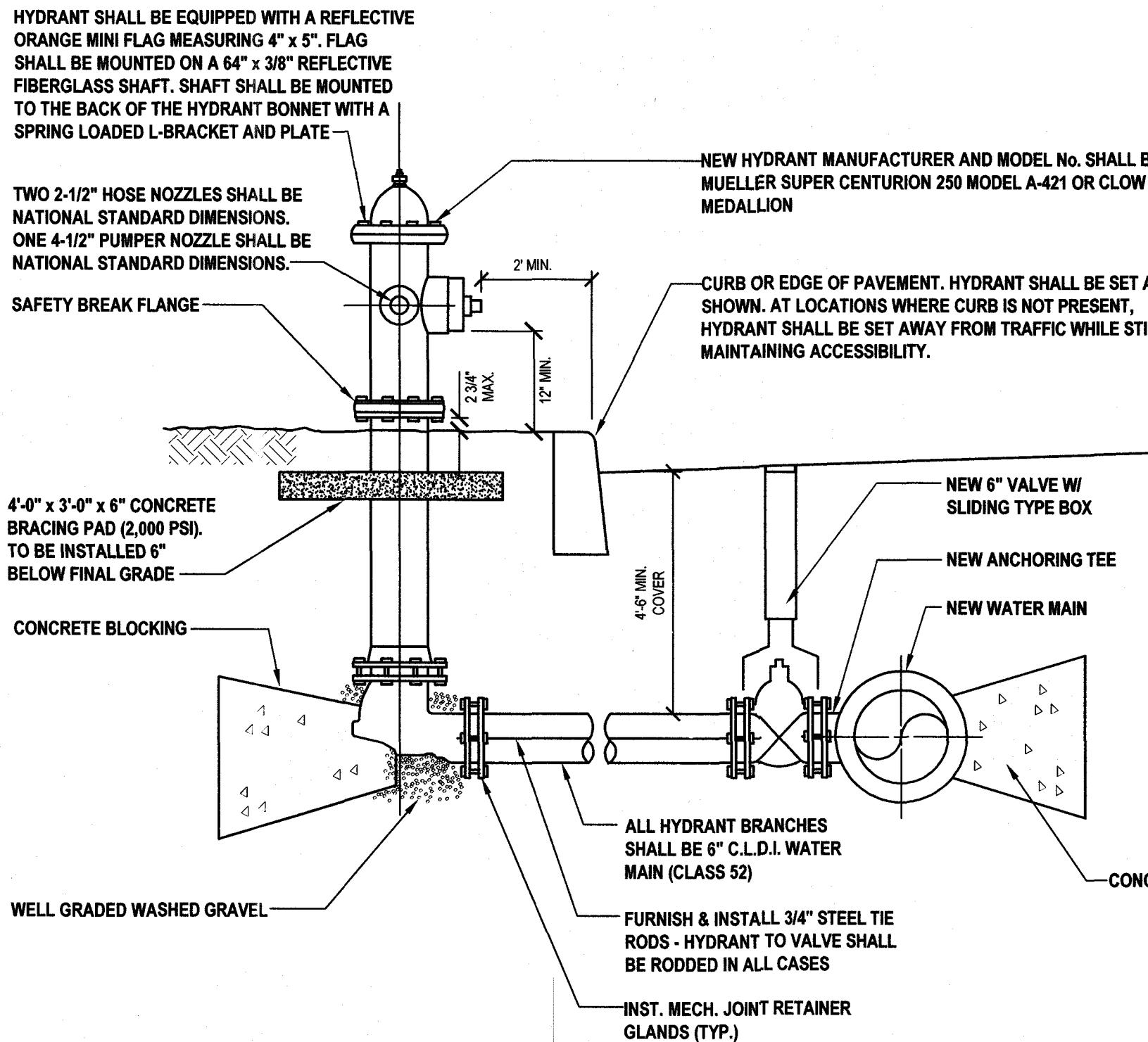
1 Typical Hydrant Installation Detail
